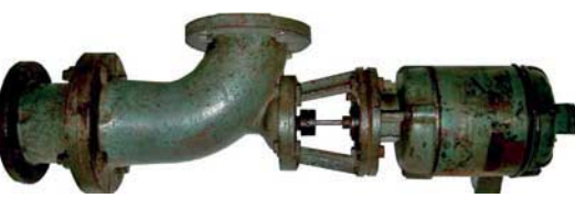
First heating circulating pump, the “elbow pump”, model year 1929, HP type DN 67/0.25 kW
